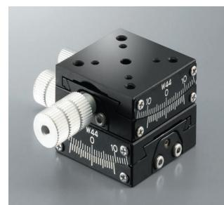
■ High cost performance goni stage which dovetail system is adapted for a travel guide, and worm gear system is adapted for feeding mechanism. Ideal for use in R&D, integrating device and much more.
