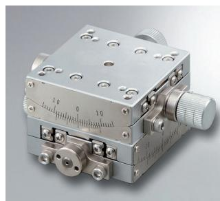
■ High cost performance goni stage which dovetail system is adapted for a travel guide, and worm gear system is adapted for feeding mechanism.
