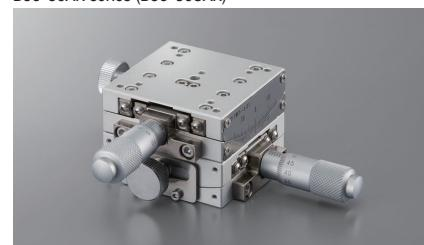
■ High cost performance goni stage which dovetail system is adapted for a travel guide, and worm gear system is adapted for feeding mechanism. Center of rotation runout accuracy is under 0.01mm(1-axis)
