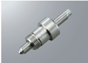
Feeding screw (Fine pitch: Handled by hex wrench) B89-2
